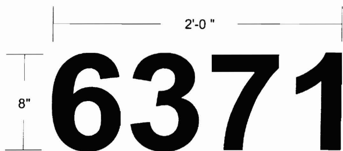
SIGNS C & E - Non Illuminated FCO "Trovicel" Letters on North Elevation (Mfr. & Install) (2 Sets Total) 1 1/2" = 1'-0"
