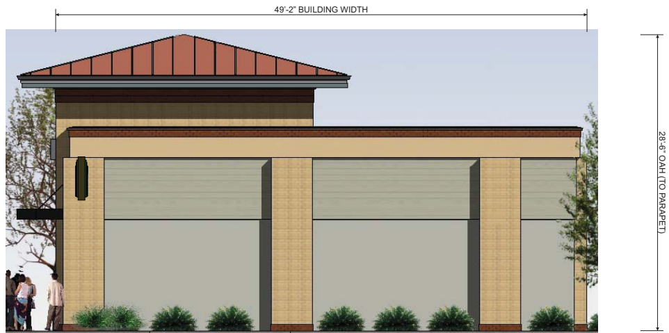
Side (Right) Elevation - Sign D 1/8"=1'-0"
