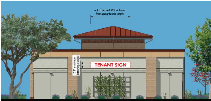
EAST ELEVATION - PAD D
