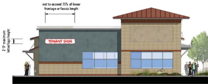
NORTH ELEVATION - PAD B
