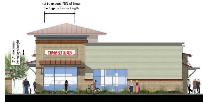
SOUTH ELEVATION - PAD C
