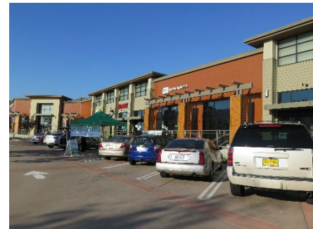
To establish a human scale along project frontages, building façades shall provide features that break up building massing at intervals of 25 to 50 feet.
